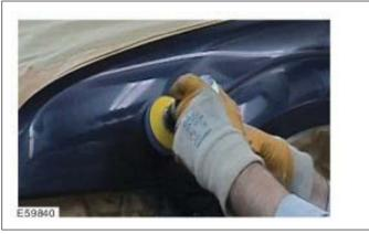
Polish the component using a polisher and polish and check the polished area for any swirl marks which may be present. Polish away any swirl marks which are present.
