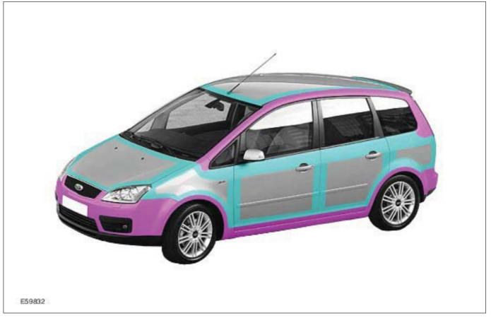
Because of their locations, the violet colored areas are the most suitable for spot repair painting. The turquoise areas are only marginally suitable and the rest of the areas are not suitable for spot repairs.
