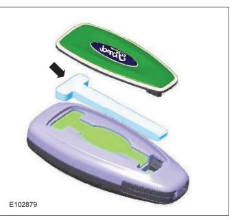
If the keyless vehicle system is unable to detect the passive key, the vehicle can be unlocked using the **emergency key**. The emergency key is integrated in the passive key.
