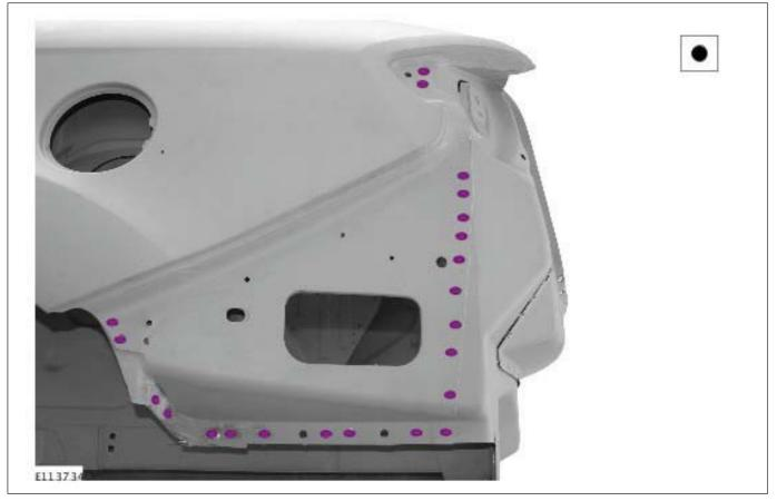
In doing so, the repair welds must match the standard of those produced in production in number and diameter.
