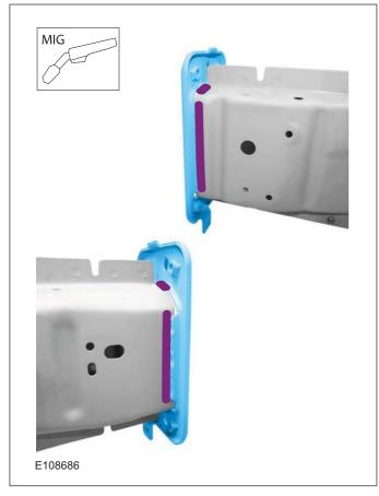
**10.** • General Equipment: Metal Inert Gas (MIG) Welding Equipment
