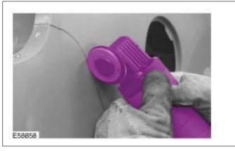
The cutting depth of the orbital saw can be set. This allows separating cuts to be made, despite panels or other components lying in danger behind. Straight cut lines can be more easily made using the orbital saw.
