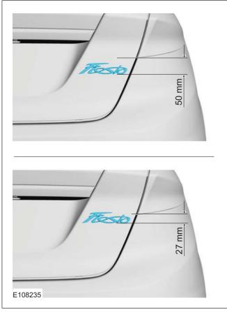
There are different positions on the vehicle depending on the vehicle specification. Before replacing, determine the dimensions from this or a similar vehicle and fit accordingly.
