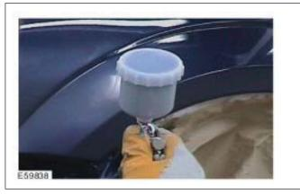
Before painting, clean the area for the final time using a dust-bonding cloth. Then apply the basic paint in thin layers using a spray gun until enough coverage is achieved.
