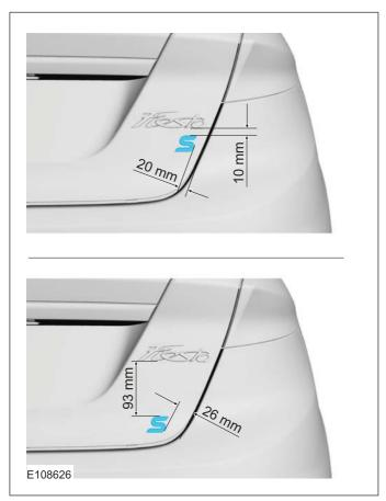
There are different positions on the vehicle depending on the vehicle specification. Before replacing, determine the dimensions from this or a similar vehicle and fit accordingly.
