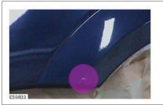
A typical case for spot repair is a small stone chip on the fender.
