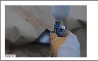
The filler layer is applied in stages. First of all, filler is only applied to the location which has been sanded away. After a wait time for flashing off, the second coat is applied so that it spreads over onto the existing paintwork.
