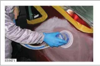
The working area is expanded by applying new masking. This makes it possible to even out the transition from the damage area to the vehicle paintwork.
