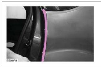
**NOTE:** Choose a suitable profile diameter. A profile which is too thick will protrude from the opening, one which is too thin will leave a gap.
