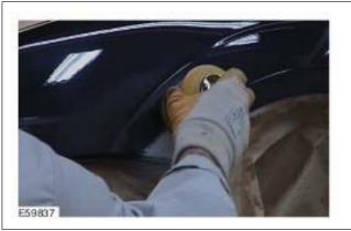
The repair location is now rubbed down with P400 - P500 and the bordering surface with P2000 - P4000. Remove sanding residues and clean the repair area with silicone remover.
