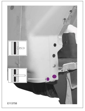
4. • General Equipment: Spot weld drill Bit
