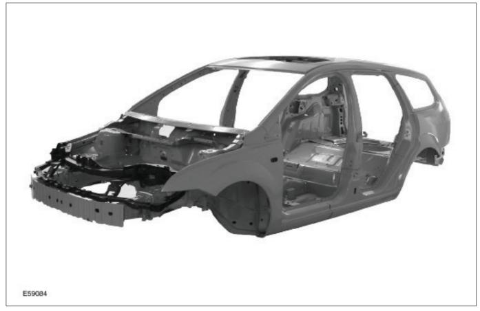
The rigidity of the bodywork is achieved by a panel skin and panel cross-section with the largest possible profile and therefore the largest resisting torque (such as for instance the rocker panel). Swage lines in the outer area of the bodywork increase the stiffness and the natural vibration frequency, to prevent possible drumming noises. The mounting points for ancillary components such as doors and wings are permanently built into the monocoque bodywork.
