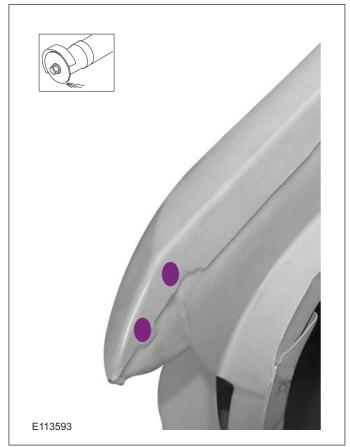
8. • General Equipment: Air Body Saw General Equipment: Spot weld drill Bit
