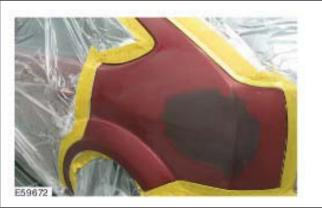
The surface which has been repaired and then prepared according to the manufacturer's instructions is now ready for basic paint application.
