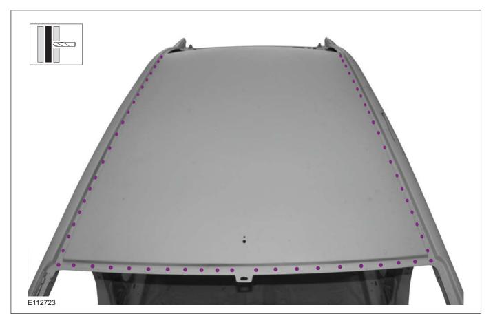
3. • General Equipment: Spot weld drill Bit
