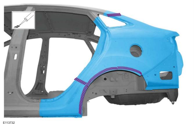
7. • General Equipment: Resistance Spotwelding Equipment General Equipment: Metal Inert Gas (MIG) Welding Equipment
