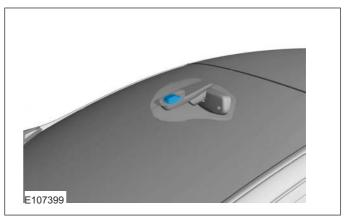
The rain sensor is built into a housing which is mounted behind the rear view mirror on the windshield. The rain sensor evaluates optical conditions. Contamination such as oil, grease or dust will prevent correct operation. Before switching on the automatic windshield wipers, the windshield must be clean in the area of the rain sensor.
