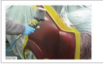
The base paint is applied in two or three steps. First of all only the repair area is painted with the first paint application.
