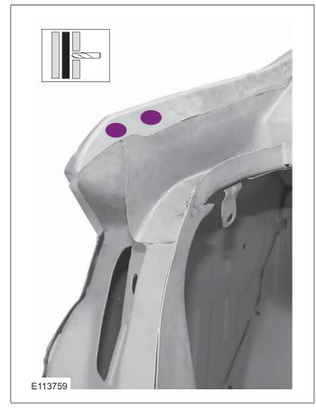
5. • General Equipment: Spot weld drill Bit
