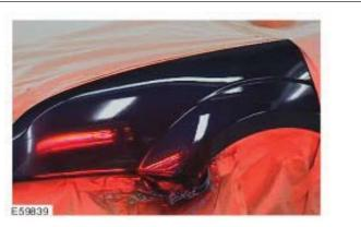
Now dry the clear lacquer according to the manufacturer's instructions using an infrared gun.
