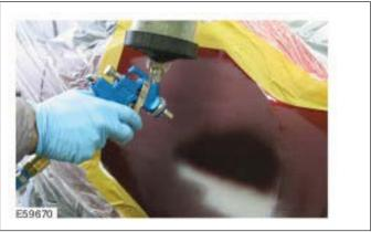
Filler can now be applied to the dried repair area. Choose the correctly toned filler according to the manufacturer's instructions.
