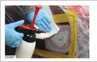
Use silicone remover to thoroughly clean the surface in order to remove grease residues, sweat from the hands and other contamination.
