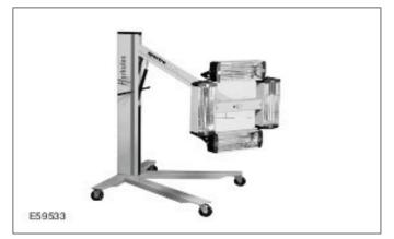
The infrared rays penetrate the air and the paint layer without warming them. Because the infrared rays are reflected from the steel panel, the paint coat is warmed from the inside outwards.
