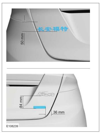
There are different variant signs and positions on the vehicle depending on the vehicle specification. Before replacing, determine the dimensions from this or a similar vehicle and fit accordingly.
