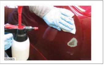
Clean the damaged surface thoroughly, to allow the extent of the damage to be seen. Use silicone remover to produce a grease-free surface.
