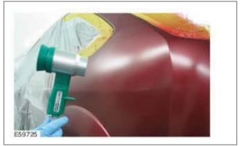
Allow the paint application to flash off until the surface has a matt appearance. So that the transition to the original paint is optimally created, the next paint application is applied to a wider area.
