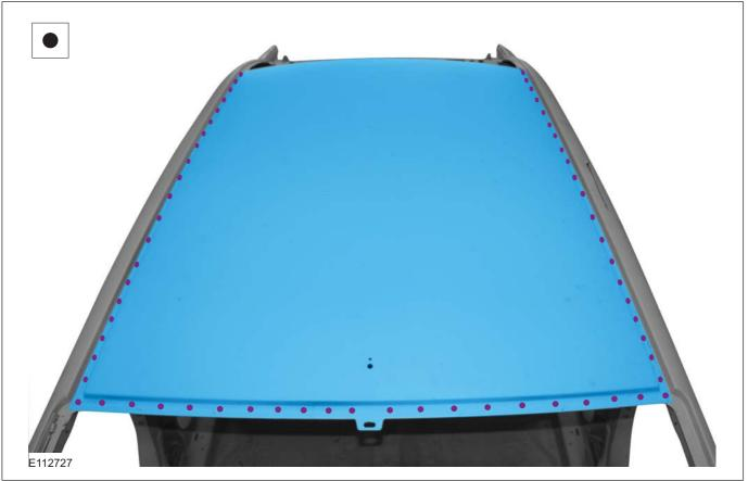
**5.** • Resistance spot weld - Panel thickness 3
