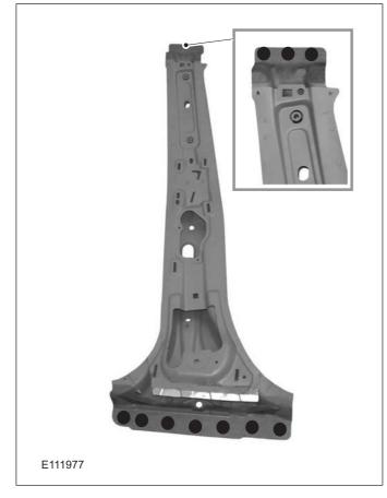
4. • A WARNING: The B-pillar reinforcement is covered with a hot-dip aluminized coating on its entire surface. This coating needs to be fully ground off on the welding flanges on the front and rear using a fibre grinding disc. Any contamination due to parts of the coating in the welding bath will weaken the welded joint.
