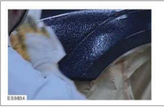
First of all the component is thoroughly cleaned using silicone remover and refurbished using abrading and polishing paste. This re-creates the original degree of shine and ensures exact color matching on the touch-up surface.
