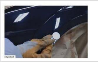
Sand out the damaged location using P180 - P320. Only small sanding blocks and small sanding machines must be used, so that the area of the repair remains as small as possible.
