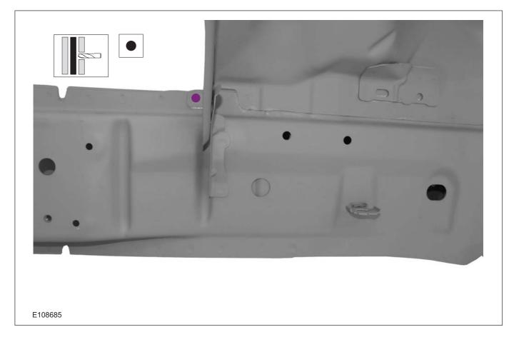
9. • General Equipment: Metal Inert Gas (MIG) Welding Equipment
