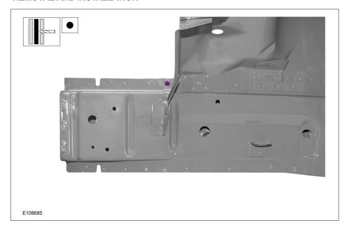
**6.** • General Equipment: Metal inert gas (MIG) welding equipment
