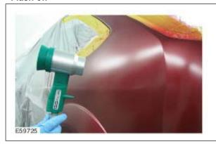
Allow the paint application to flash off until the surface has a matt appearance. So that the transition to the original paint is optimally created, the next paint application is applied to a wider area.
