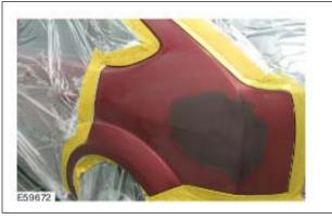
The surface which has been repaired and then prepared according to the manufacturer's instructions is now ready for basic paint application.
