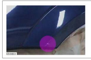
A typical case for spot repair is a small stone chip on the fender.
