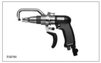
In contrast to a normal drill, the milling depth can be set. This prevents the underlying panel from being damaged. In addition a safety fixing system prevents the milling cutter from slipping while working.
