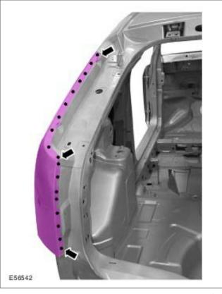
The repair welds must have the same number of weld spots as the welds used in production with the correct diameters.
