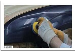
Polish the component using a polisher and polish and check the polished area for any swirl marks which may be present. Polish away any swirl marks which are present.
