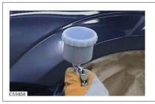
Before painting, clean the area for the final time using a dust-bonding cloth. Then apply the basic paint in thin layers using a spray gun until enough coverage is achieved.
