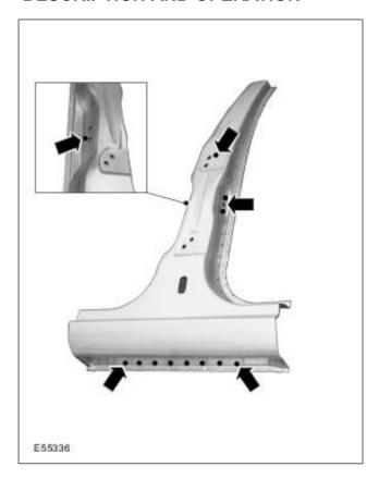
component is shown in dark green. Spot welds, weld seams and cut lines are shown in black.
