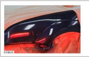
Now dry the clear lacquer according to the manufacturer's instructions using an infrared gun.
