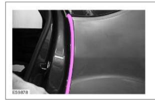
**NOTE:** Choose a suitable profile diameter. A profile which is too thick will protrude from the opening, one which is too thin will leave a gap.
