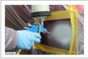
Before applying stopper, apply primer to the sanded and bare surface.
