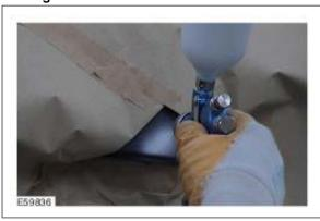
The filler layer is applied in stages. First of all, filler is only applied to the location which has been sanded away. After a wait time for flashing off, the second coat is applied so that it spreads over onto the existing paintwork.
