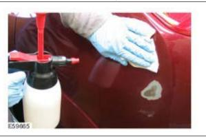
Clean the damaged surface thoroughly, to allow the extent of the damage to be seen. Use silicone remover to produce a grease-free surface.
