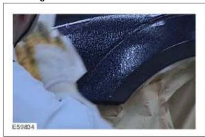
First of all the component is thoroughly cleaned using silicone remover and refurbished using abrading and polishing paste. This re-creates the original degree of shine and ensures exact color matching on the touch-up surface.
