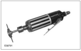
It is also suitable for releasing MIG spot welds and MIG seam welds.
