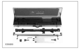
By the use of two parallel laser heads which can be turned, symmetrical points of a vehicle body can be tested and compared. Using the linear scales which are attached to the measuring points, the measurement data is read off with the aid of the projected laser beams.
