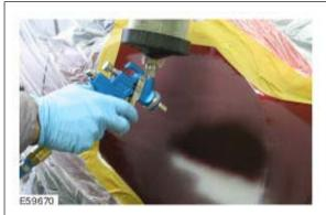
Filler can now be applied to the dried repair area. Choose the correctly toned filler according to the manufacturer's instructions.
