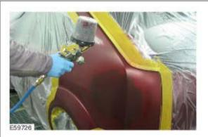
The base paint is applied in two or three steps. First of all only the repair area is painted with the first paint application.
