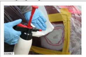
Use silicone remover to thoroughly clean the surface in order to remove grease residues, sweat from the hands and other contamination.
