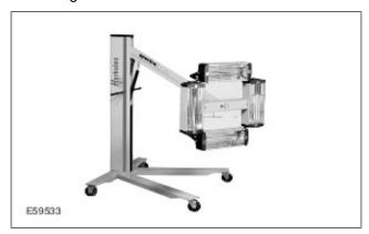
The infrared rays penetrate the air and the paint layer without warming them. Because the infrared rays are reflected from the steel panel, the paint coat is warmed from the inside outwards.
